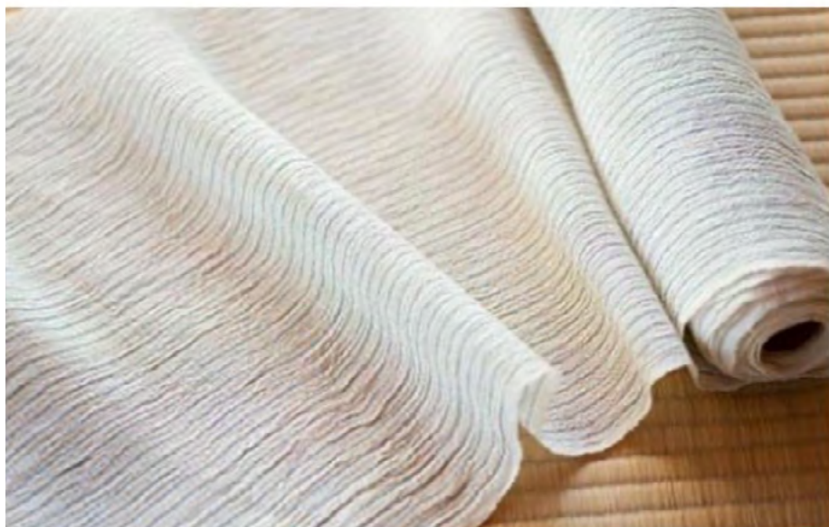
Figure-3. A stretch fabric made using silk yarn as warp and paper yarn as weft. [Courtesy: Kokusai Pulp & Paper Co., Ltd. [11].
