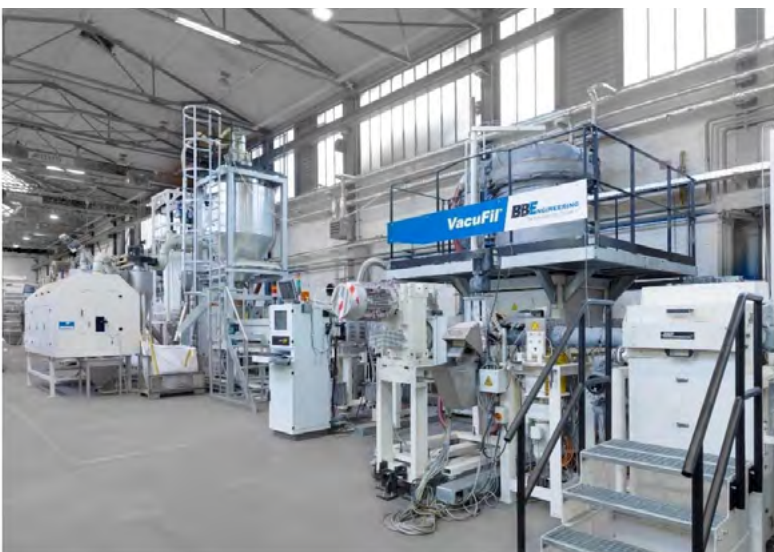
The VacuFil test system at the company HQ in Remscheid is available for customers and interested parties for material and process testing.
